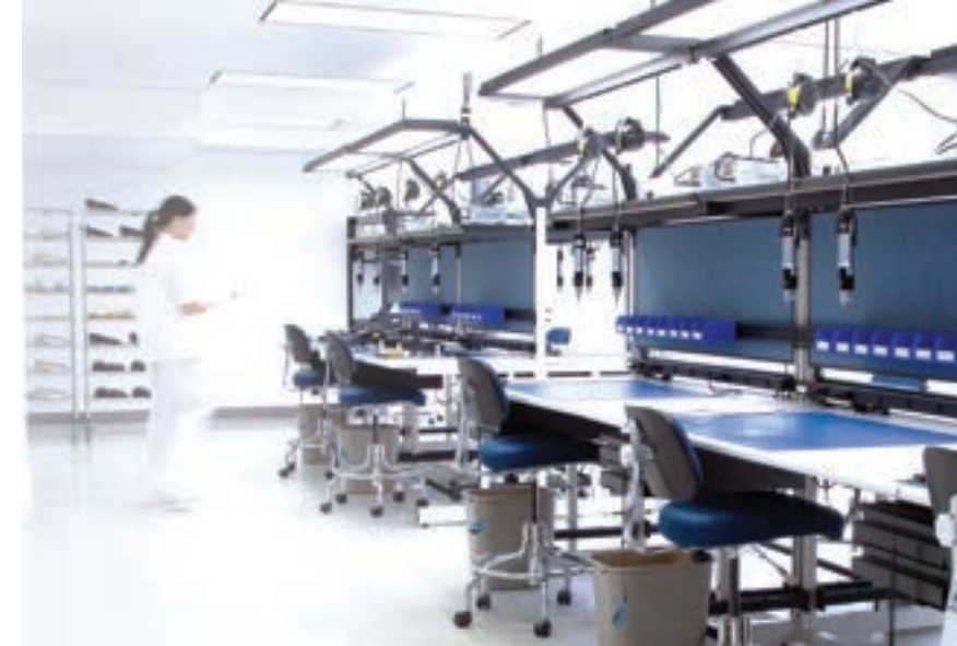
Every medical-grade foot control we manufacture is built in our Medical White Room, which features ESD Safe Construction for handling electronics, such as anti-static pads, grounded chairs, and grounding bracelets for technicians.
