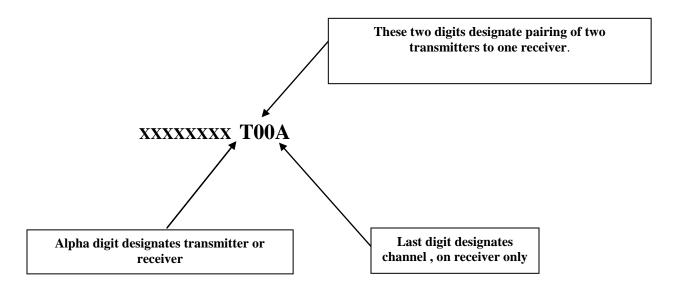
In addition to the 15 channels each manufacturer has its own code encryption. This assures that different manufacturers with the same channel marking can be used in the same area simultaneously with no interference. The manufacturers code is embedded into the model number as shown below. It also appears on a label on the top of the units.
